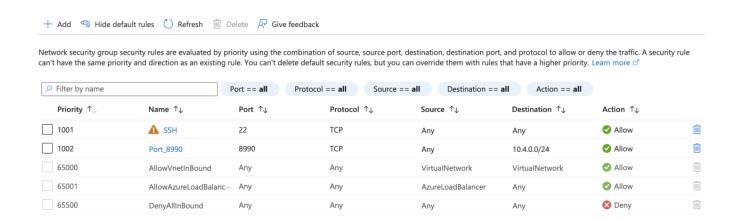
Fig. 1.3: Example compute nodes inbound security group rule
