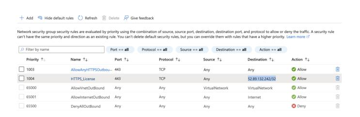
Fig. 1.4: Example compute nodes outbound security group rules
